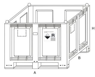
The CARGOPALLET 600 NEW PLUS is available in the version approved for land and rail transport and for the storage of solid dangerous products in compliance with ADR regulations. The container is equipped with a string and an identification label showing the 4 types of batteries that can be stored: UN 2794, UN 2795, UN 2800 and UN 3028. Equipped with two bars on the long side, it is versatile and robust, with excellent rigidity structural and resists deformation.
