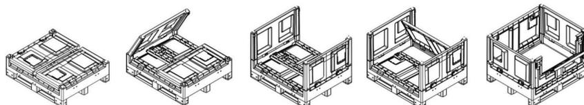
Cargo Fold 700 with runners is completely folding. With this system, in case of transport and storage of empty containers, you shall earn 63% in volume: a stack of eight folded Cargo is the same height as three open ones.
