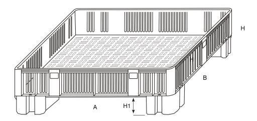
The new CARGOPALLET 280 has been specifically designed to store and to transport food and vegetables. Made by injection moulding of high density polyethylene, non-toxic material for foodstuff, it is a stackable container with perforated sides and base.
