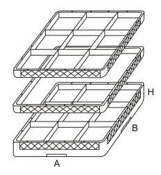
BASKETS have perforated walls that ensure better washing and perfect drying, with the reduction of limestone formations.
