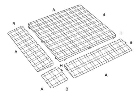
A full surface modular floor system that guarantees perfect adherence to the surface. Also available in self-extinguishing and conductive versions. Rated operational voltage 3 kV. It comes complete with a side and corner joint for even more functional floor paving.
