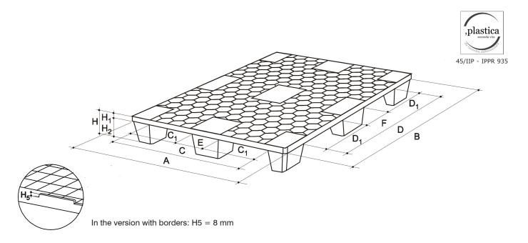
The My-A 600x800 pallet, which is half the size of the standard dimensions, as the name implies, are rendered far more robust and solid by their totally new concept of honeycomb structure, which makes them ideal for intensive use.
