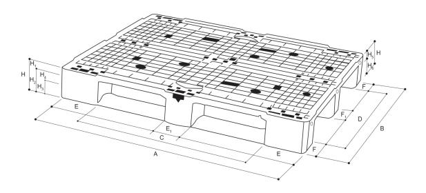
The Pallets My-E are specially designed for heavy load. The loading plate and the sleepers are moulded in one piece. The sleepers are perfectly vertical and are ideal for automatic handling and storage. The pallet can be supplied with or without perimeter borders. Thanks to its grilled structure, it is easy to clean and at the same time impermeable to liquids.
