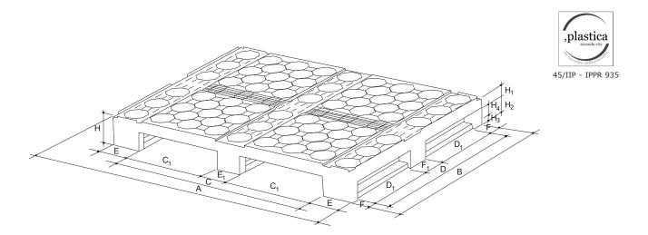
The PALLET My-P 600x800 for heavy loads, has the floor with a honeycomb geometry surface that facilitates cleaning .The robust beams allow for intensive use even heavy loads on racks.
