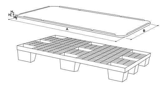
The flat for pallet is totally closed and smooth, adapts to all 800x1200 pallets. It can also be used as top / cover for goods loaded on a pallet. The containment edges are purposely interrupted to accommodate the strap.
