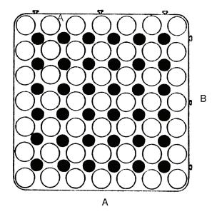
The self-modular Sigma elements made of special green shockproof resin are particularly suitable for flooring in graphic and mechanical industry as they can absorb to a great extent the vibrations produced by plants, and dampen the relevant noises.
